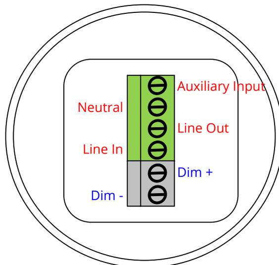
Diagram above shows the screw connector terminals of Lantern Dimmable occupancy sensor. It has one high voltage connector and low voltage connector. High voltage connector is green in color and has four terminals. Low voltage connector is grey in color and has two terminals. In the high
