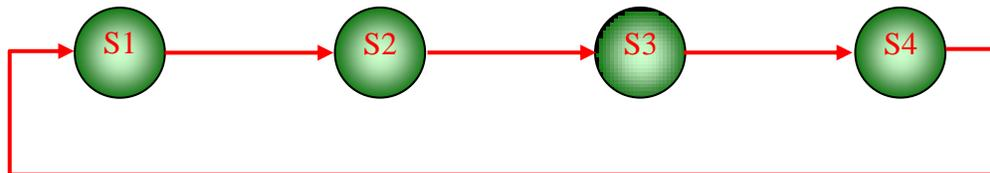
chain; no sensor is head or tail. When S1 detects occupancy, it will switch ON the load connected to all the sensors. Similarly when S4 detects occupancy, it will switch ON the load connected to all the sensors including the one connected to S1.
