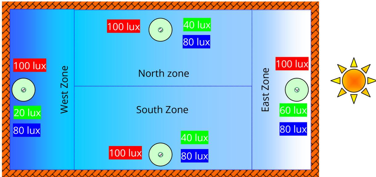
zones and are connected to dimmable luminaries. With conventional sensors, each of these zones will receive, about 80 lux from artificial light in order to meet the minimum light requirement for the west zone. As a result, there is 20 lux extra lighting in the south and north zones while 40 lux extra light in the east zone. So there is a potential for additional energy savings.
